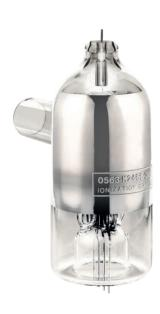
The 563 is a rugged gauge with wide range of linear response:  $2 \times 10^{-10}$  to  $1 \times 10^{-3}$  Torr. The platinum coating inside the bulb shields the gauge elements from electrostatic charges at low pressures and drains off the static charges which can build up at high pressures. The 563 is available in a variety of tubulations.
