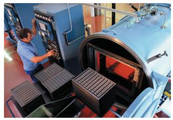
Plasma vapour deposition (PVD). Worker adjusting the controls of a PVD machine which is being used to coat components (trays at lower centre and lower left) with a thin film metal alloy to provide a wear-resistant coating.
