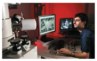
Scanning electron microscopes, like the one shown here, can "see" details as small as one nanometre – one millionth of a metre!
