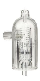
The 571 offers high performance and wide range (2 x  $10^{-10}$  to 1 x  $10^{-3}$  Torr). The gauge is rugged; it can withstand long periods of degassing or accidental exposure to atmosphere at operating temperature and still recover its original characteristics.
