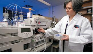
An NRC researcher uses a liquid chromatography-mass spectrometry system to quantify toxins in shellfish samples.
