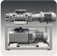
2009-2010 Innovative line of TPS Turbo Pumping Systems. New High Capacity MS Rotary Vane Pumps and RPS Roots Pumping Systems, for demanding industrial vacuum applications.
